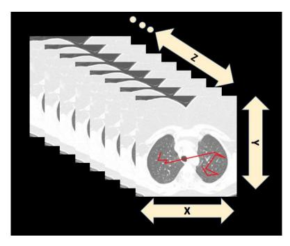
**Figure 1.** Eye tracking in 3D stacks of images means keeping track of the eye's position in the XY plane and the depth (Z) of the currently displayed image.
